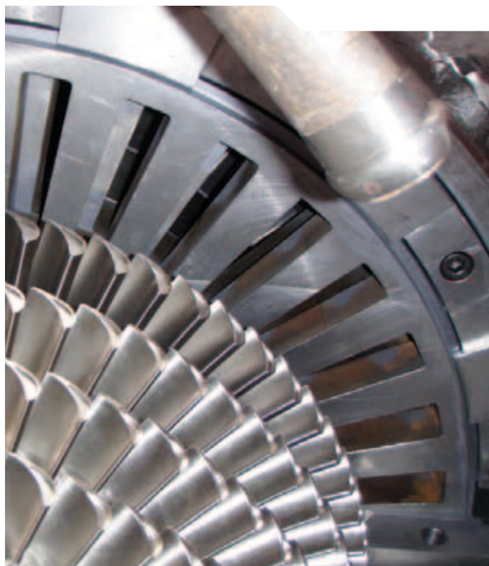
Swivelling control diaphragm of a extraction condensing turbine
