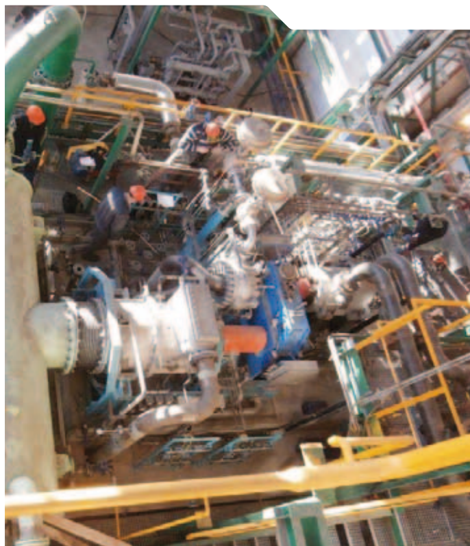
Steam condensing turbine driving a hydrogen compressor
